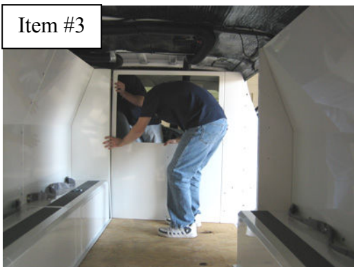
Attach Front Bulkhead to Driver-side Bench/Wall assembly
